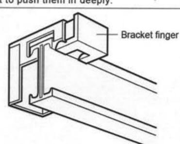
3 Detach the rail from the brackets, and cut away any excess portion with a cutter or hand saw.
