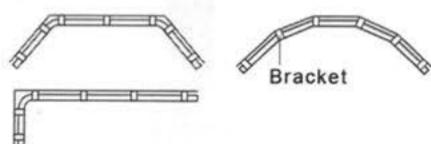
Temporarily attach the rail to the fixed brackets at the end, and determine the rail length.
